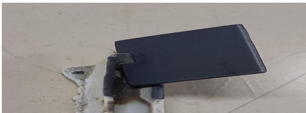
Fig -3 : Copper and Alumina crucible taken out of the muffle furnace
