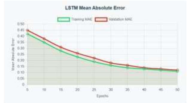
Fig. 5. LSTM mean absolute error progression showing consistent reduction to final validation MAE of 0.12, indicating precise severity predictions.
