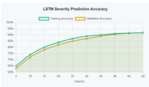
Fig. 4. LSTM accuracy over 50 epochs showing stable convergence around epoch 35 with 91.8% validation accuracy and robust temporal pattern learning.
