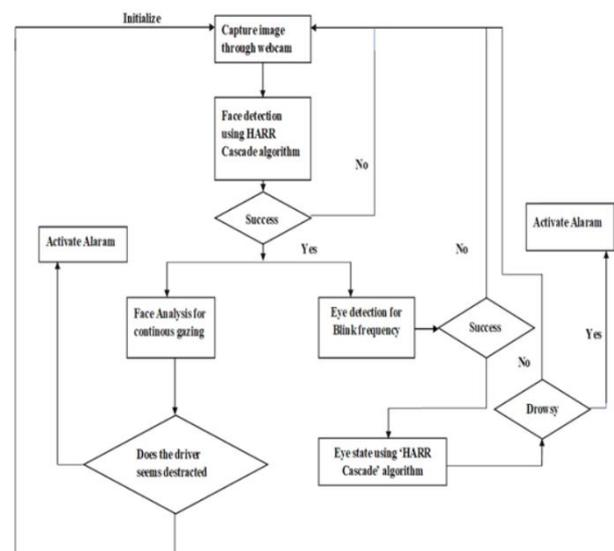
**Fig.2: Flow Chart of Driver Safety Enhancement System Using Arduino and Buzzer Alert**
