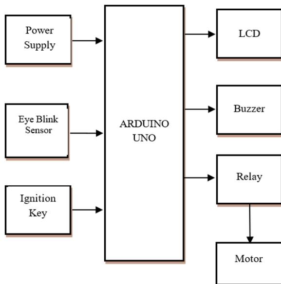
**Fig.1: Block diagram of Driver Safety Enhancement System Using Arduino and Buzzer Alert**
