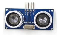
Fig. 5.1 (e) Ultrasonic sensor
