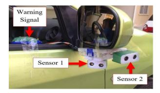
Fig. 8.3 Blind spot installation for on-road testing
