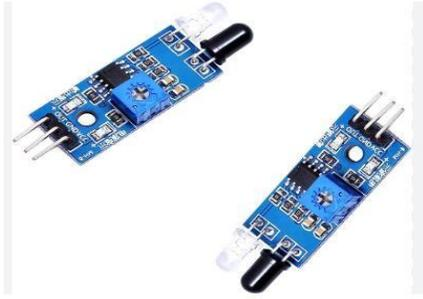
Fig. 5.1 (f) Infrared Sensor
