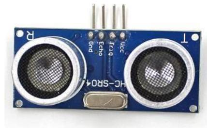
Fig. 5.1 (e) Ultrasonic sensor
