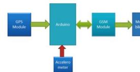
Fig. 6.1.4 Block diagram for accident indication
