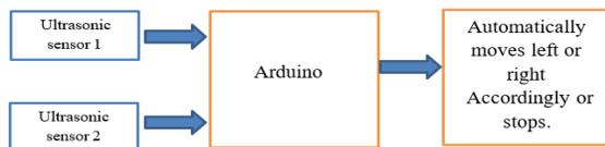
Fig. 6.1.1 Block diagram for Blind Spot Detection
