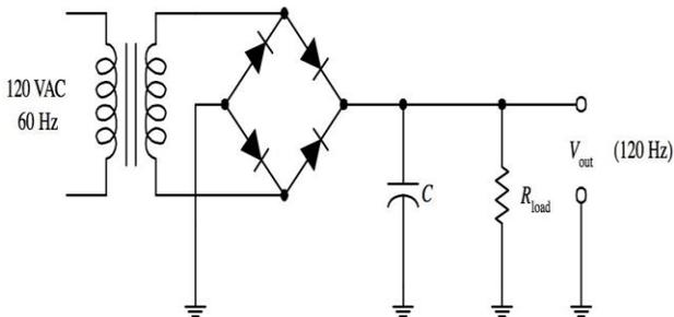
Fig. 5.1 (a) Circuit diagram of Power supply
