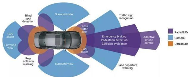
Fig. 7.1 Advantages of Driving Control Systems in car
