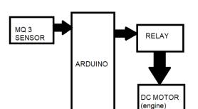
This above block diagram is for the alcohol detection system. In this firstly the alcohol state of driver is detected using the MQ3 sensor. This sensor monitors the alcohol rate in the air within the driver range. If the alcohol rate is high then this sensor sends signal to the arduino chip as it is connected to the sensor. This arduino chip controls the motion of the vehicle using relay which is connected to the braking system of the vehicle.
