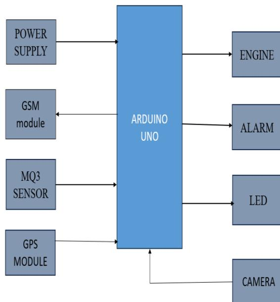
Fig 4.1 Block Diagram
