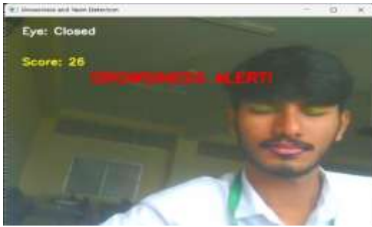
Fig 4 : Detection of Eye Closure
