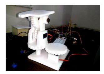
Fig 2: Prototype of Dual-axis solar tracker.
