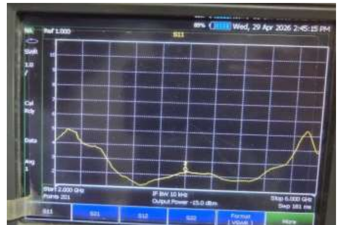
Fig. 7. Experimental validation results: (a) Return loss ( S_{11} ) vs frequency, (b) VSWR vs frequency.
