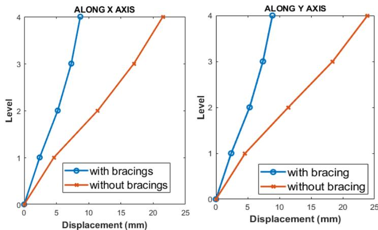
Fig.6 Average displacements of the with and without steel bracings
