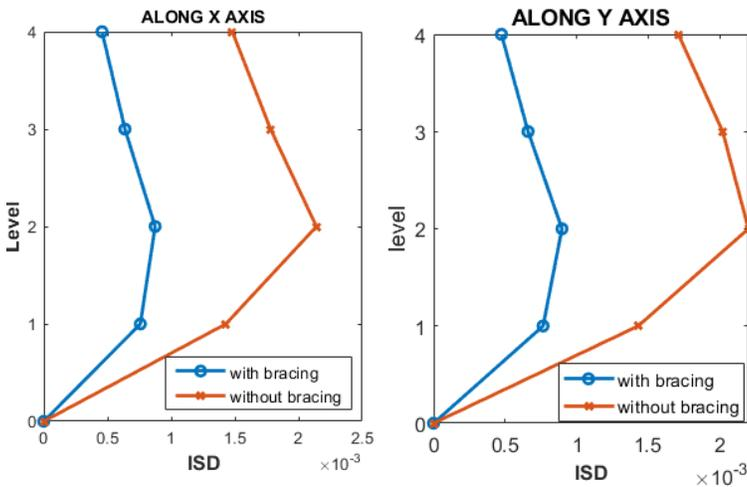
Fig.4 Average ISD for with and without bracing frame in both direction
