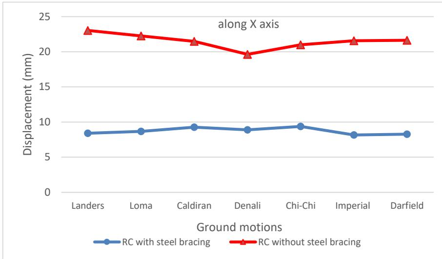
Fig.5 Maximum displacement of the selected ground motions along with the x directions
