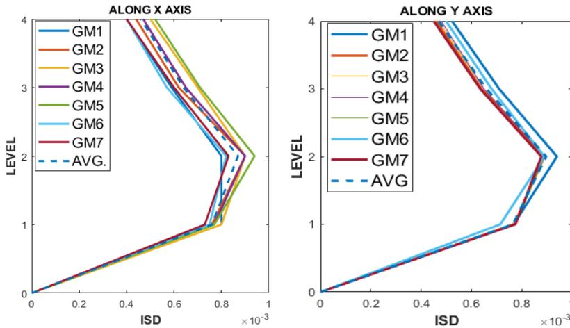
Fig.3 Inter story drift (ISD) of four-story with steel bracing (retrofitted) building in both direction
