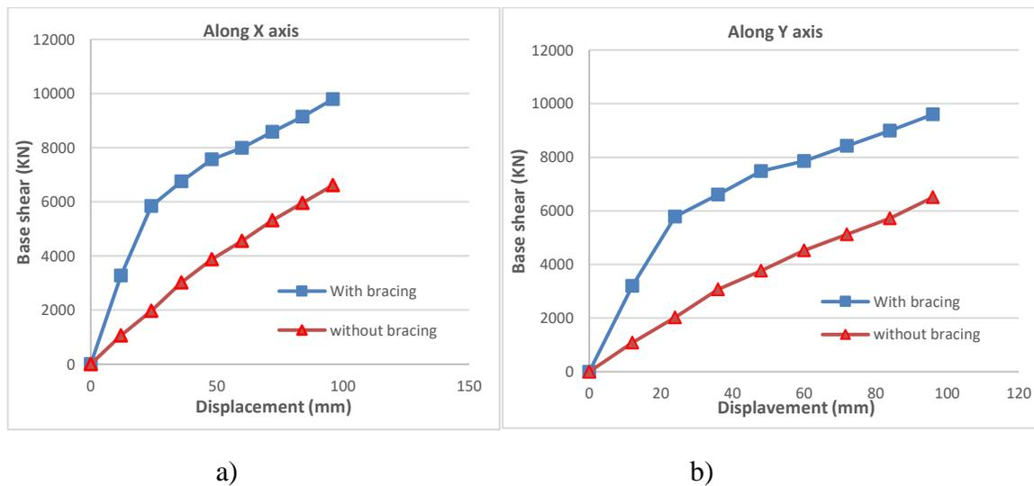
Fig. 2 Capacity curves for 4 story structures, a) along the x axis, b) along the y axis.
