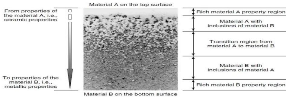
**Figure 1.1 Gradation of an FGM**
