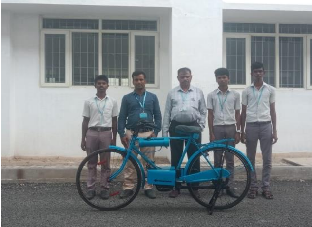
Figure 3 Final 2S Engine fitted bicycle . The motorized bicycle is slight weight and
