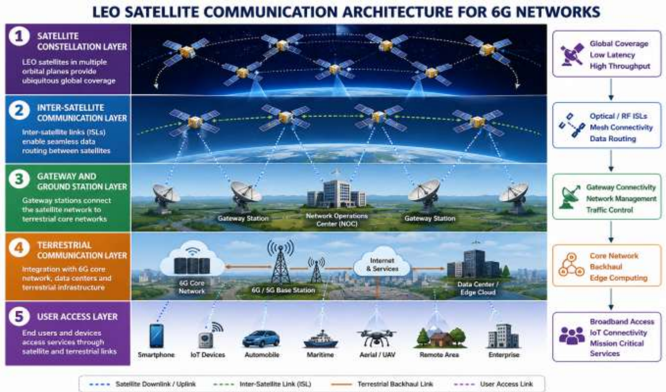
Fig 1 A typical LEO satellite communication architecture for 6G networks
