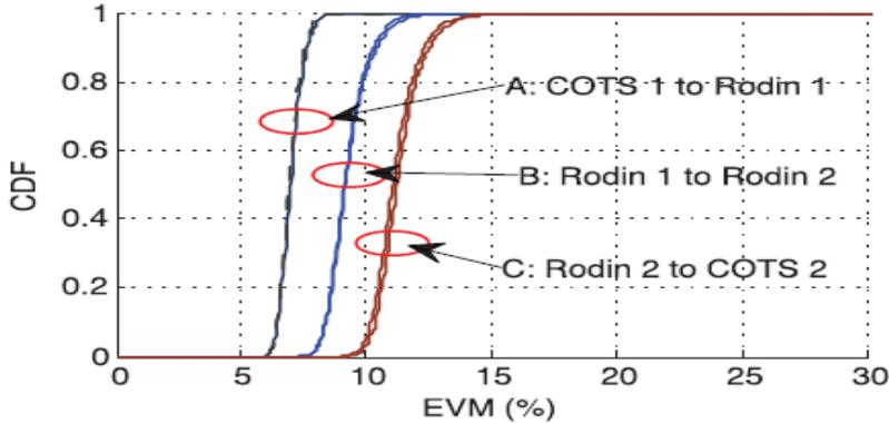
Figure 5. EVM of symbols in an OFDM frame with and without spectrum shaping.
