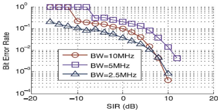
Figure 6. BER of OFDM frames measured at COTS 2 without shaping.
