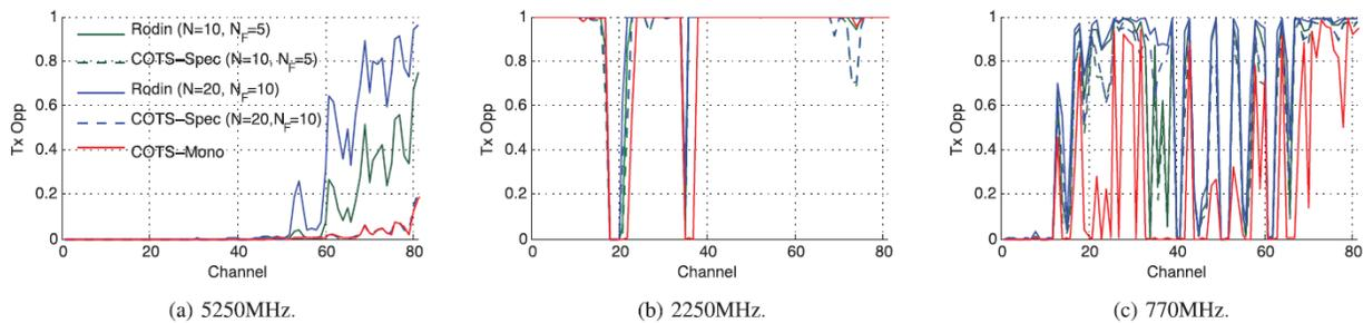
Figure 7. Proportion of time slots that each of the devices, RODIN, COTS-Spec, and COTS-Mono, can transmit in.
