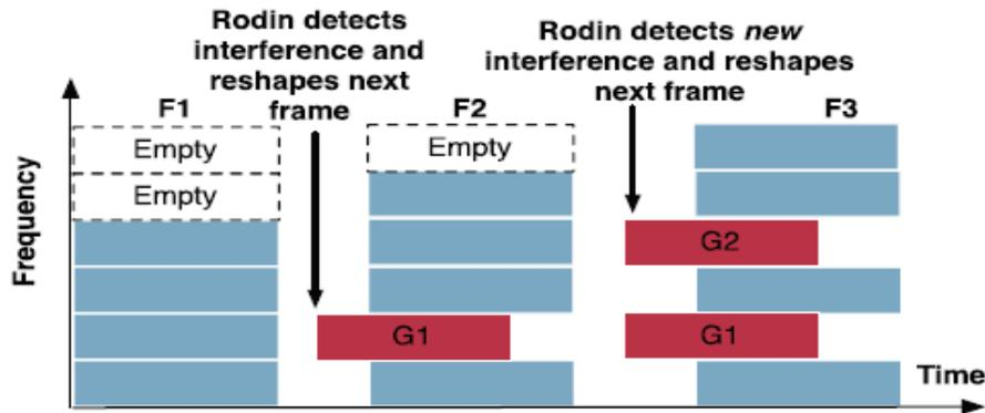
Figure 1. Transmission of three frames.
