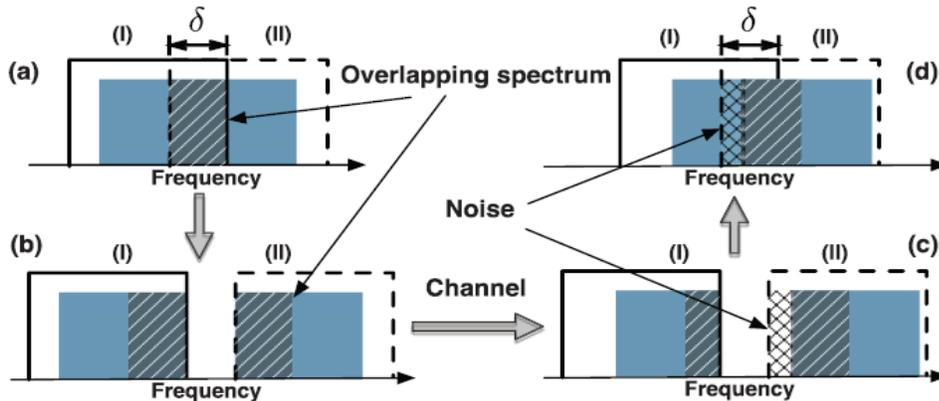
Figure 2. Spectrum shaping using two partially overlapping filters.
