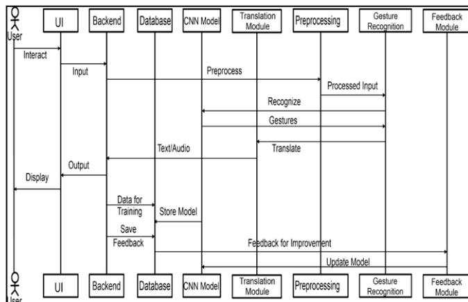
Figure 2. System Architecture.
