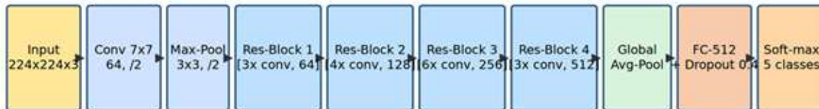
Figure 2. Architecture of the ResNet-50 backbone with the custom classification head used in this study.
