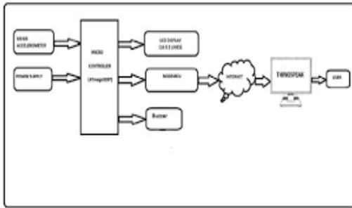
Fig.2 Block diagram of require earthquake alert system
