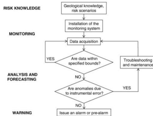
Fig 3. Flow chart of working of an earthquake alert system
