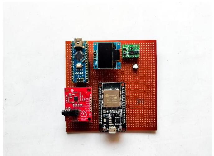
**FIG 1: ECG Monitoring system with oximeter**
