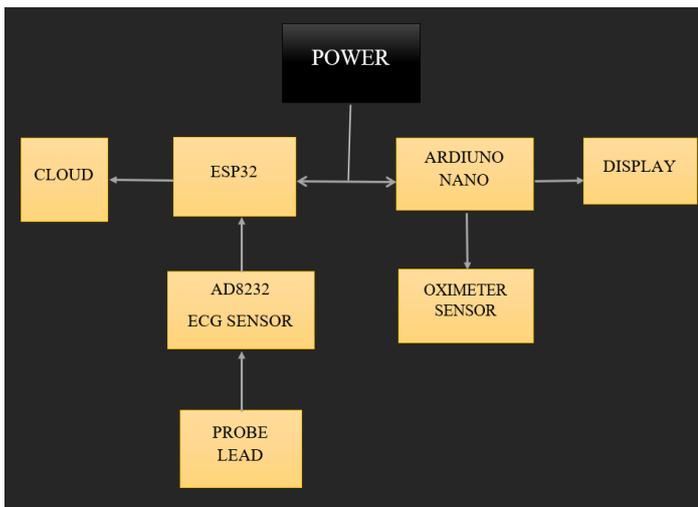
**Block diagram: ECG Portable Monitoring system**
