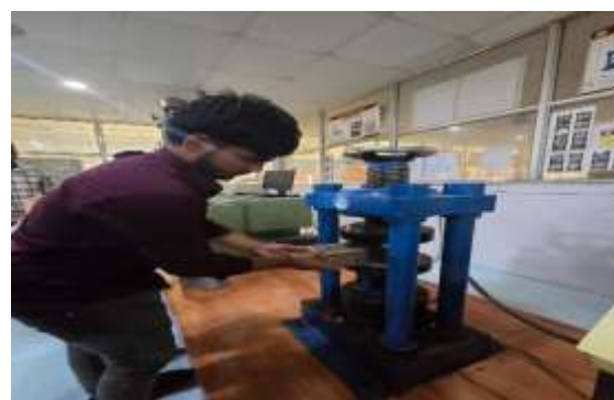
Fig 5: Compression Test on Cow Dung Brick
