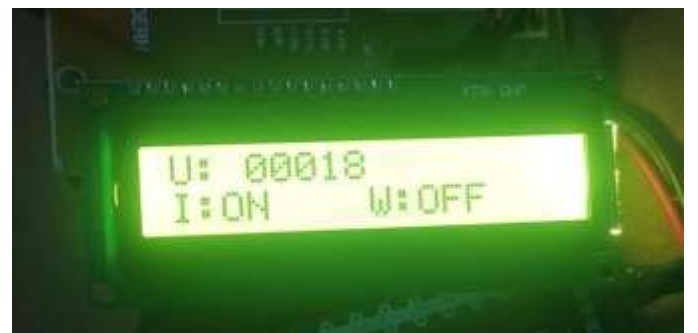
Fig: 4.12. Display Update I: ON — indicating dry (inorganic) waste detected.
