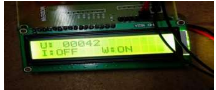
Fig :4.10. Status Update on LCD W: ON — indicating wet waste has been detected
