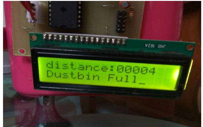
Fig 8.1 Smart bin equipped with LCD display and sensors
