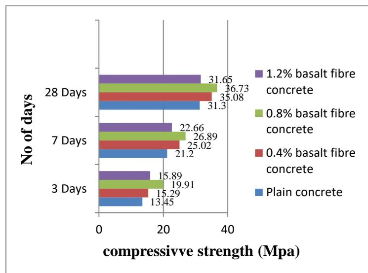
**Graph 1 Plain Concrete Vs.0.4, 0.8, 1.2% Basalt Fibre Concrete**
