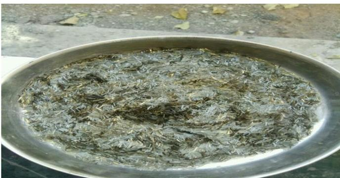
**Figure 1- Chopped Basalt Fibre**
