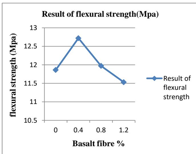
**Graph 2 flexural Strength At 28 Days (Mpa)**
