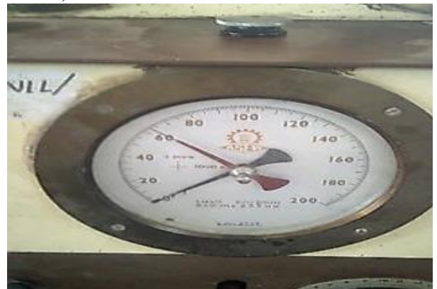
Fig. 6. Machine indicator needle (Point of failure).
