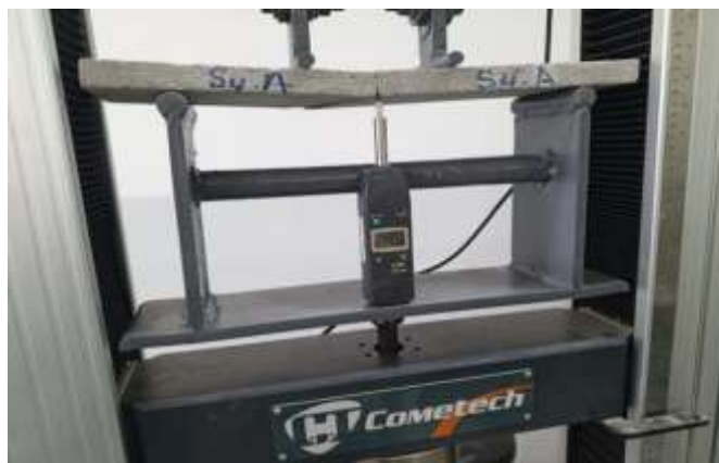
Figure 3. Testing of flexural strength using LVDT.
