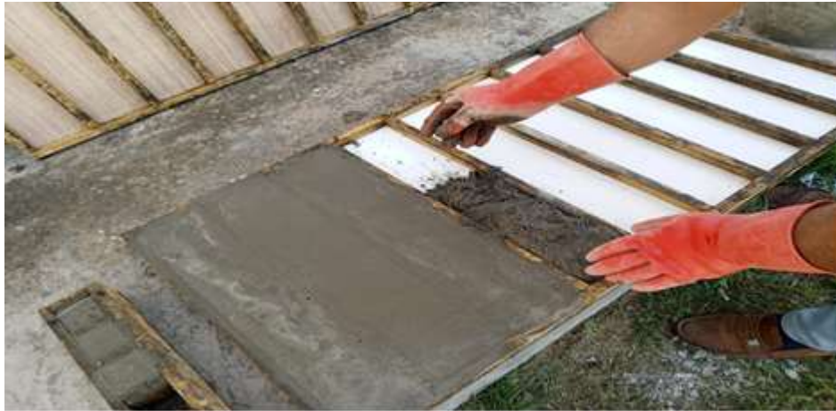
Figure 2. Casting cubes and beams.
