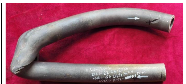
Fig. 1 Failed Platen Superheater Tube superheaters and reheaters, operating at high steam
