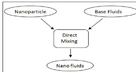
Fig.4.2 One step method to prepare Nanofluids.
