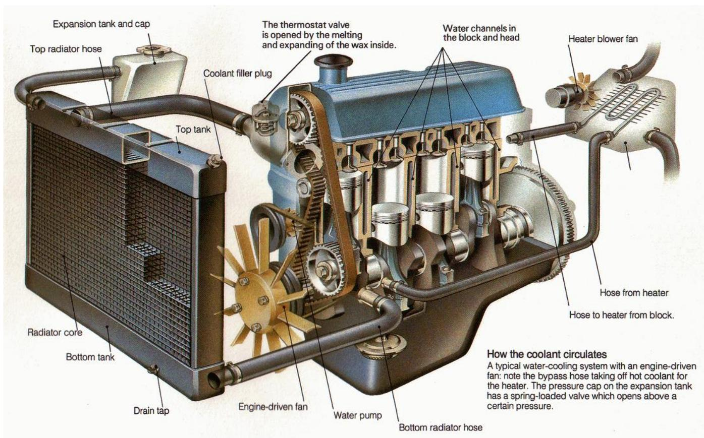
Fig. 2.1 Engine-Radiator Assembly
