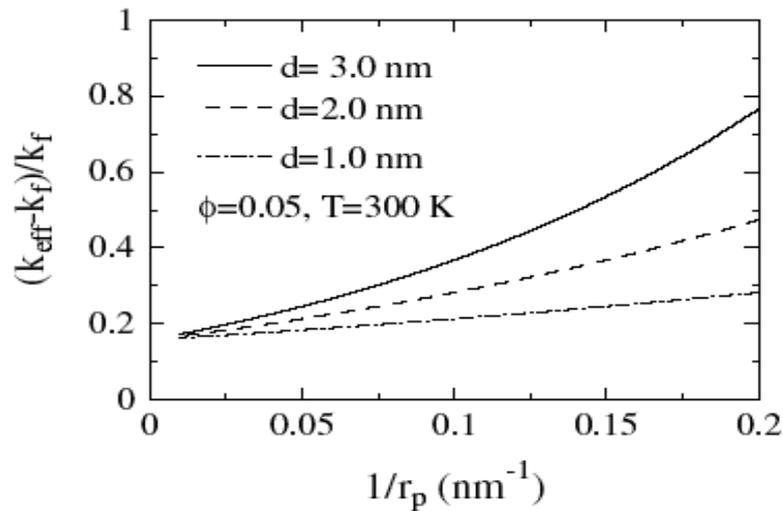
Fig.1.1 Dependence of thermal conductivity enhancement on Oxide/water Nanofluid on the reciprocal of the nanoparticle radius.
