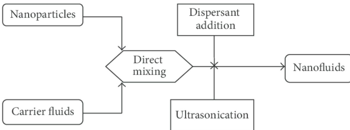
Fig.4.1: Two step method for preparing Nanofluid
