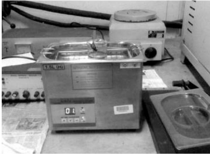
Fig.6.1: Sonication as a method of Dispersion
