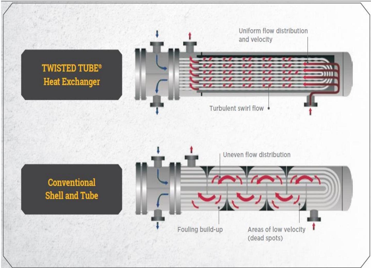
Fig.1.2 Comparison between twisted tube and conventional heat exchanger
