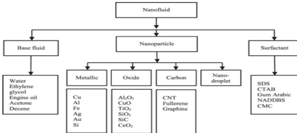
Fig.4.4: Preparation of Nanofluid (Tabulated View)
