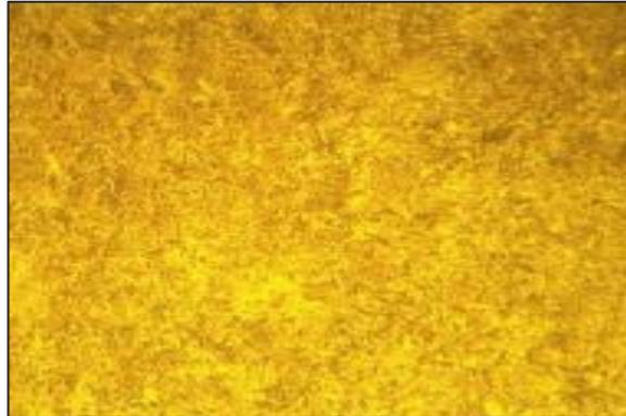
**Figure 4 : Microstructure of hardening & tempering EN24**
