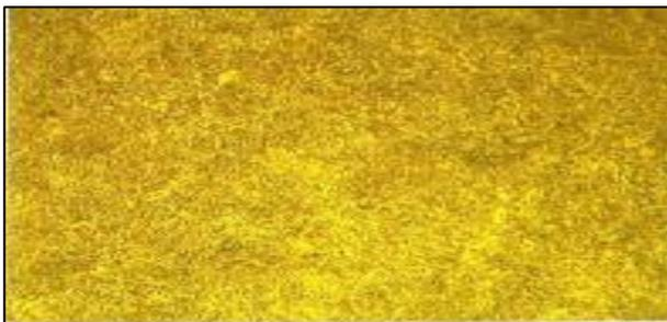
**Figure 2 : Microstructure of Annealing EN24**
