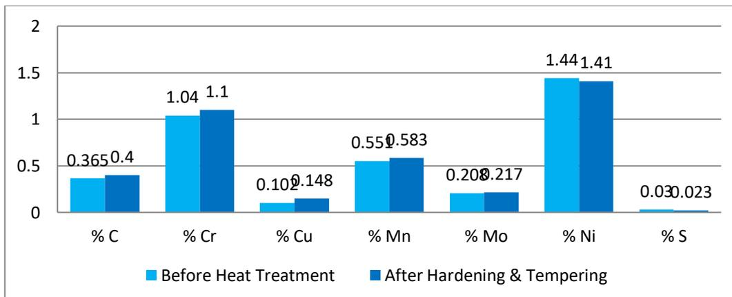
**Fig .8 Variation of chemical composition percentage for before and Hardened & Tempering specimens.**
