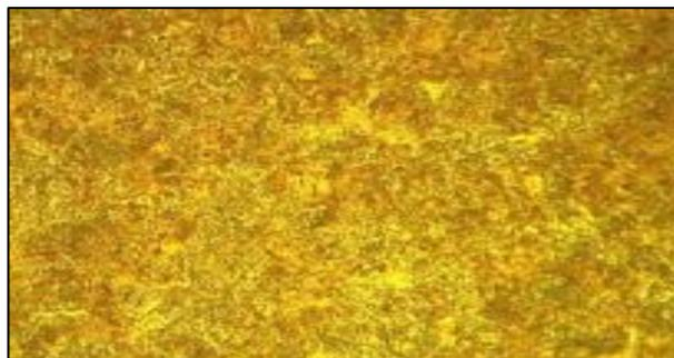
**Figure 3 : Microstructure of normalizing EN24**
