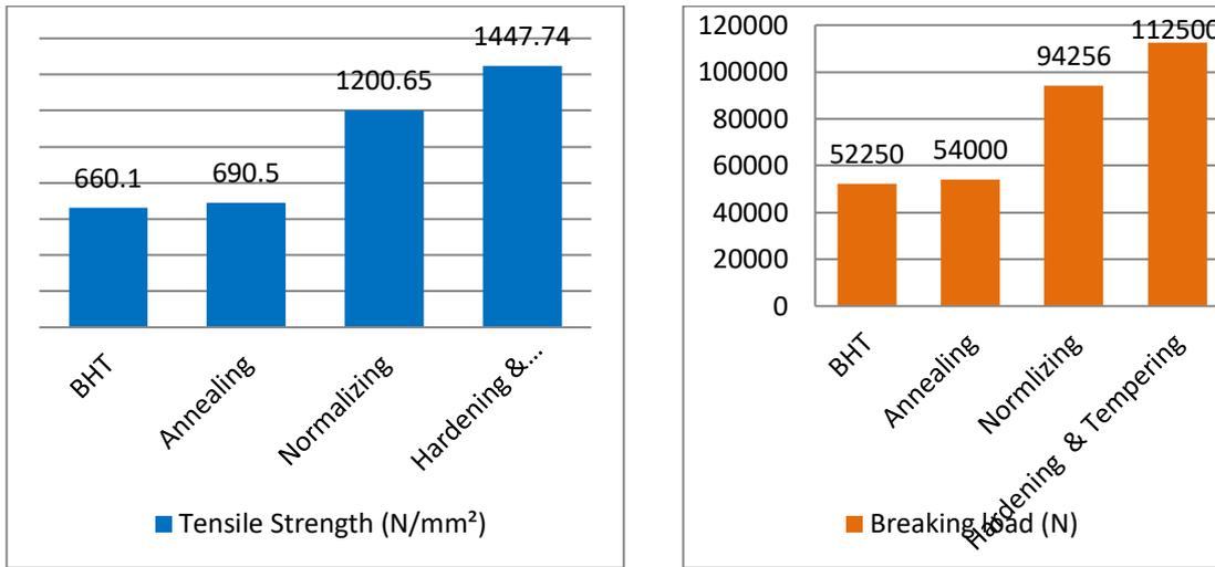
**Fig 6 (a & b). Tensile strength and Breaking load variation due to different heat treatment processes**
