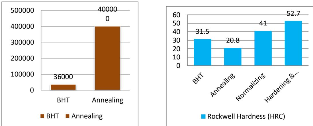
**Fig 7 (a & b). Variation of hardness and Yield load variation due to different heat treatment Processes**
