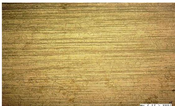
**Fig 4 Microstructure after Quenching**
