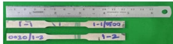
**Fig 2 Tensile Test Specimen before Quenching**
