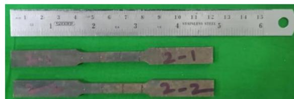
**Fig 3 Tensile Test Specimen after Quenching**
