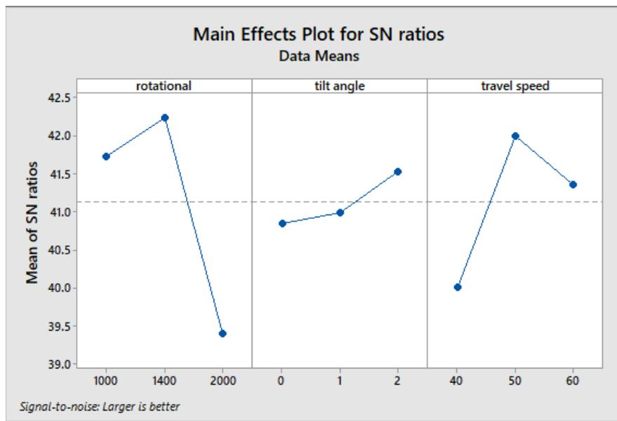
This graph shows that variation of means of mean with respect of process parameters
