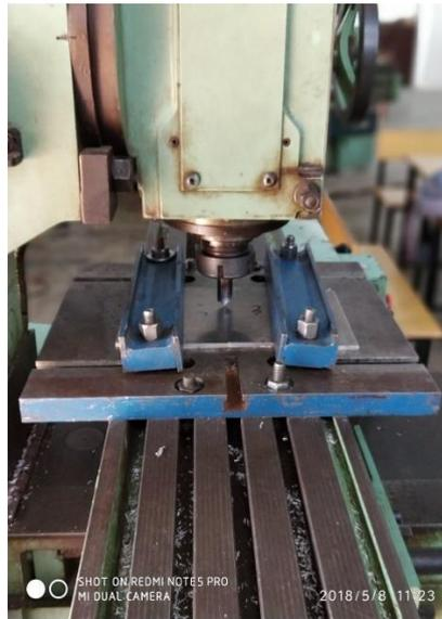
Vertical milling center machine used as friction stir welding machine setup.
