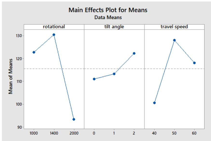
The above graphs show the main effect plotted against mean values for various outputs and using percentage contribution. Here it shows that the tool rotation speed is the main factor to be effectively decided with the contribution ratios as mentioned in the above ANOVA table. From the above graphs maximum hardness is observed at travel speed of 50 mm/min, the Tool Rotation speed of 1400 rpm, and tilt angle of 2.
