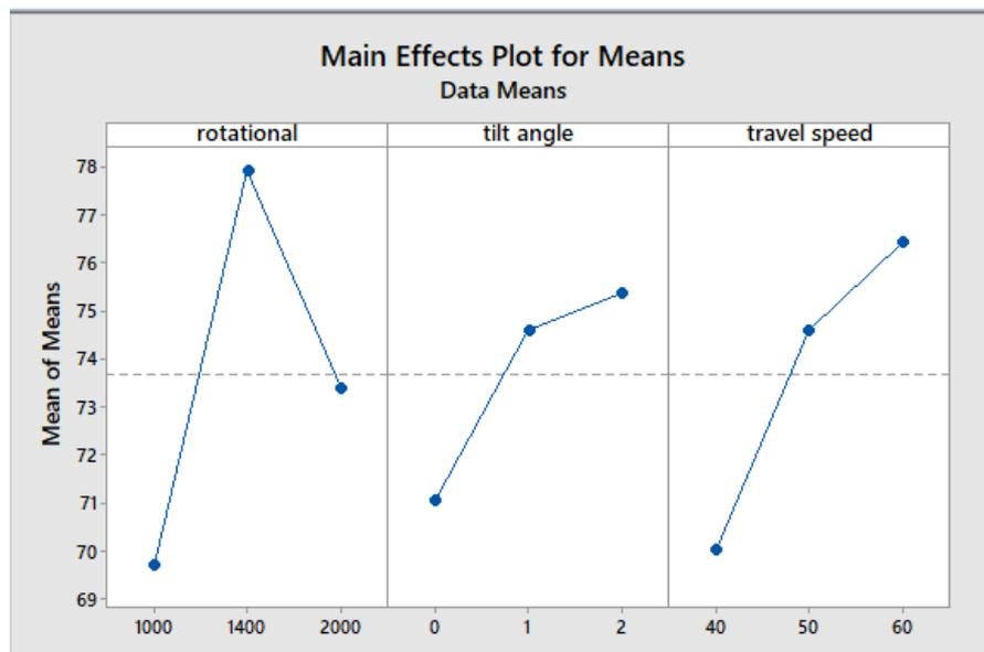
The above graphs show the main effect plotted against mean values for various outputs and using percentage contribution. Here it shows that the tool rotation speed is the main factor to be effectively
