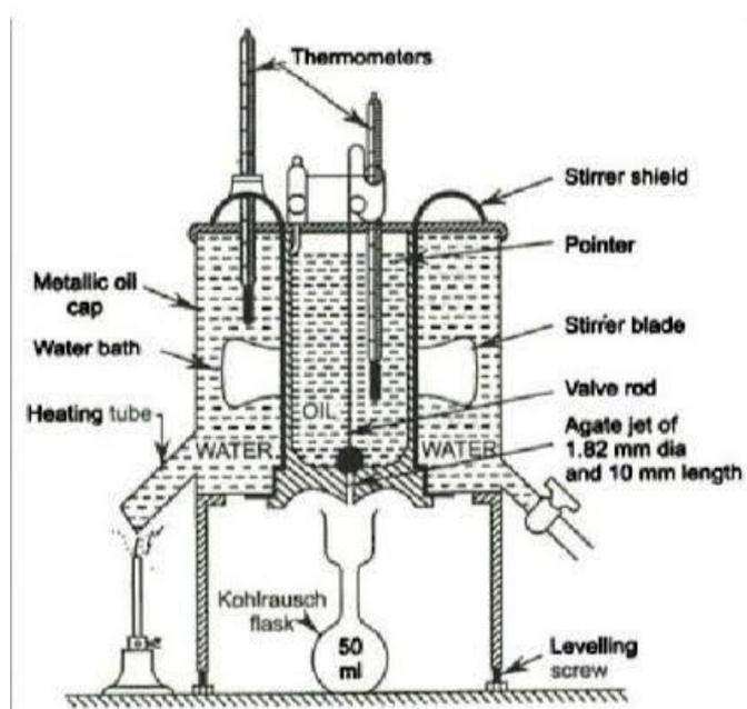
**Figure 1** diagram for Red Wood Viscometer
