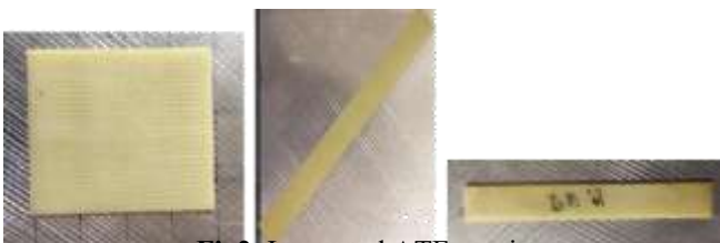
Fig2. Immersed ATF specimen taken out from furnace after 7 days
