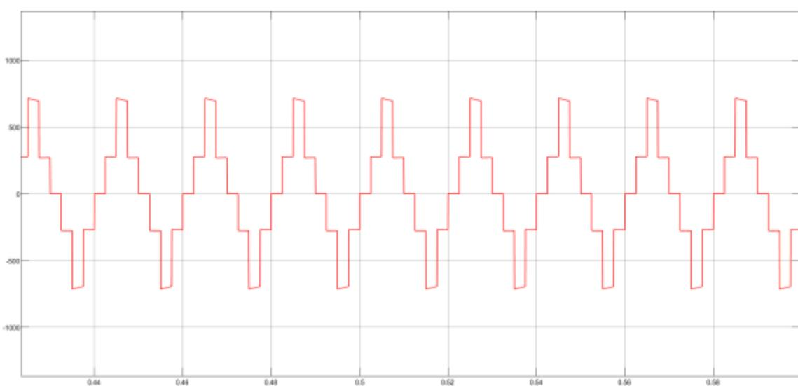
Fig – 6. 5-level inverter output waveform
