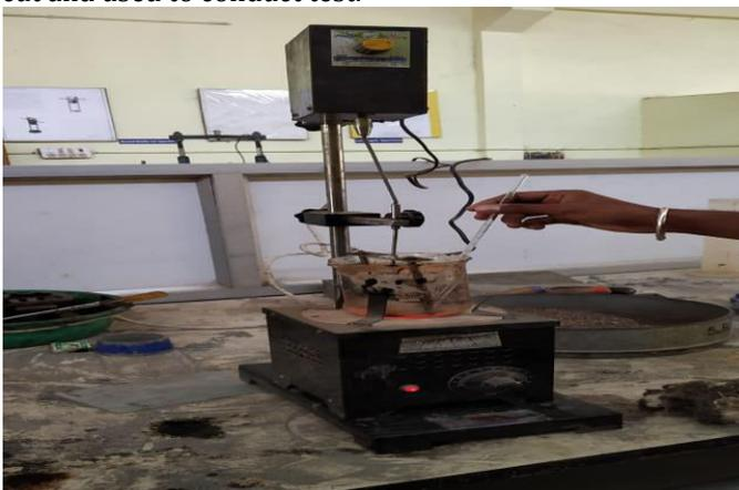
Fig -6: Softening Point Test
