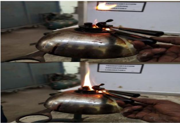
Fig -5: Flash and Fire Point Test
