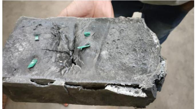
Fig -4: Failure Pattern of Paving Block under UTM
