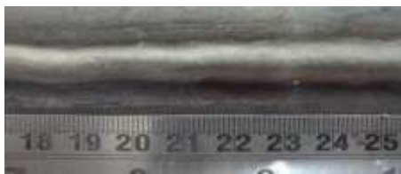
Figure 1(a): Hardfaced layer- Sample-1
