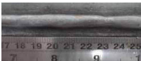
Figure 1(c): Hardfaced layer- Sample-3
