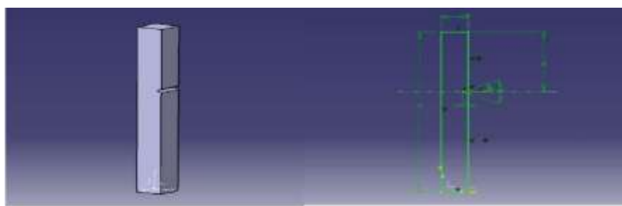
FIG.4.Isometric view of specimen for Izod impact test
