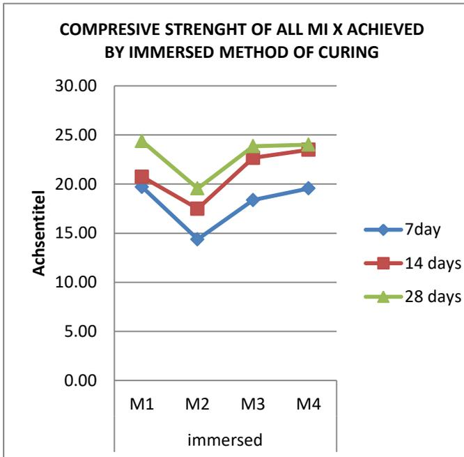
Chart 1 Compressive Strength Achieved By Immersed Technique for Curing
