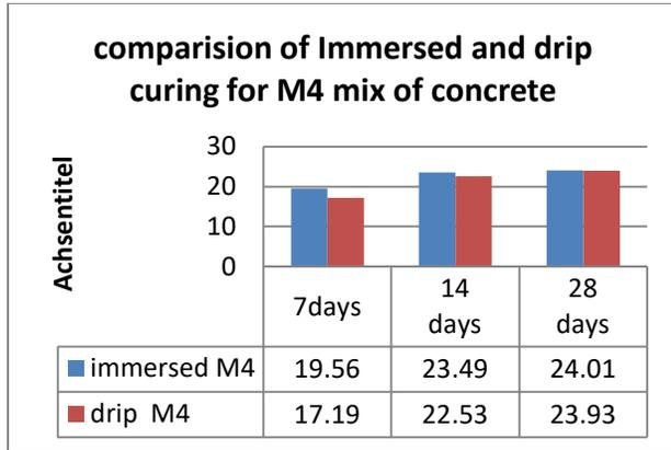
Chart 4: Comparison Of Immersed and Drip System for Mix 4
