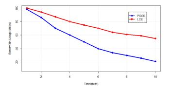
Fig 2: Average Bandwidth utilized by PSGR and LCE algorithms
