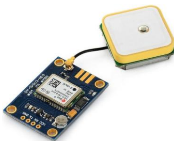
Figure 3: GPS Sensor with patch antenna
