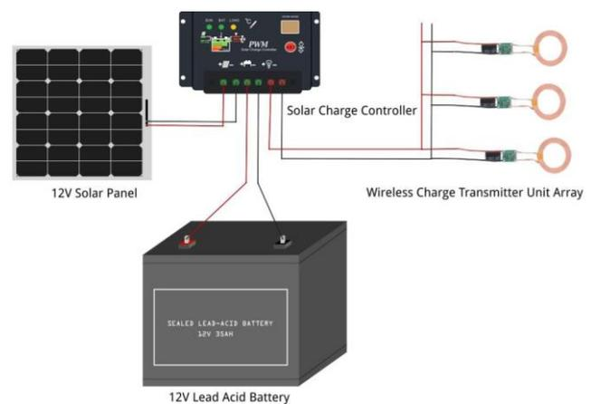
Figure 2: Circuit Diagram of Road part
