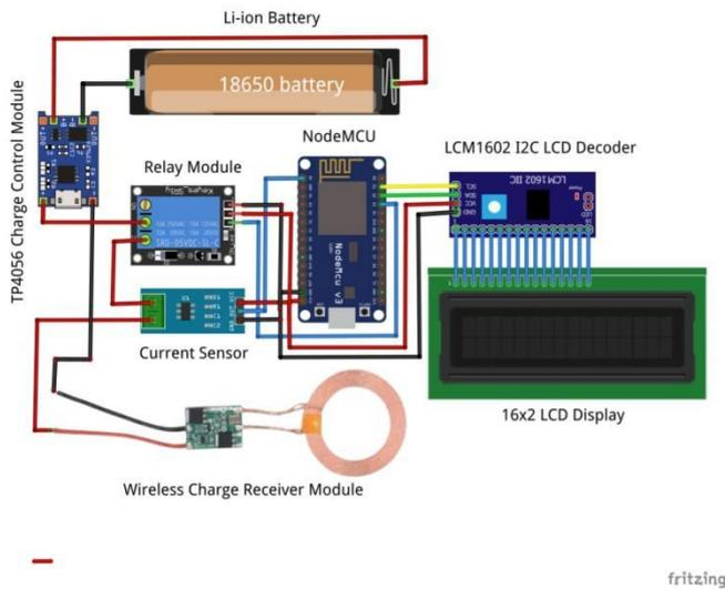
Figure 3: Circuit Diagram of Car part
