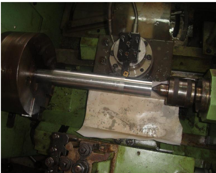
Fig 3.2: Tool, dynamometer and W/P assembly
