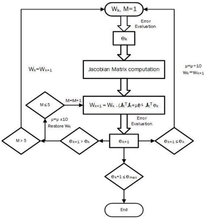
Fig. 1: Block diagram for training using Levenberg–Marquardt algorithm
