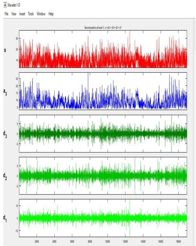
Fig. 6: Wavelet decomposition up to level 3 of wind speed.
