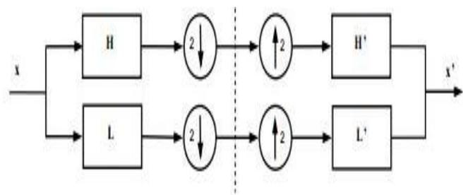
Fig. 3: Filter Bank Scheme for DWT
