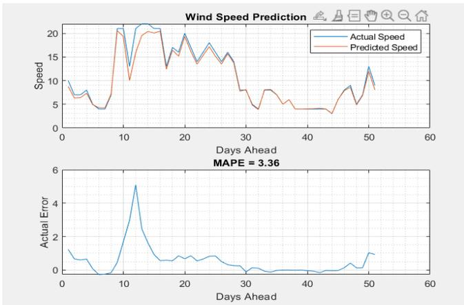
Fig 8: Comparison between the predicted and actual wind speed employing the proposed model using back propagation
