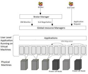
Figure1: System View of Cloud Environment
