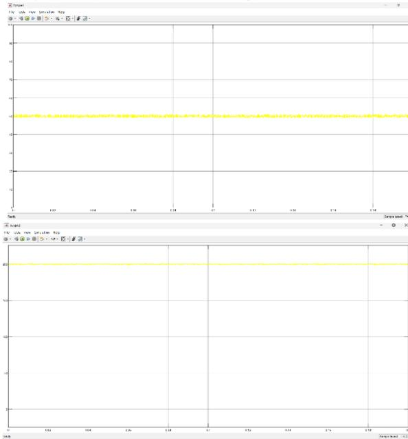
FIGURE 9. Controlling the DC-link voltage's dynamic aspects: (a) The voltage of the DC-link if the load current decreases (b) Voltage of the DC link with a rise in load current.
