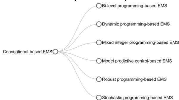
Fig. 7: Types of conventional-based optimization techniques used in EMS
