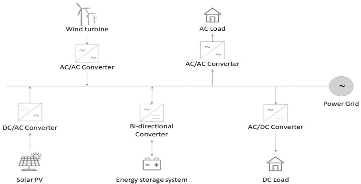
Fig. 3. Grid-Connected Microgrids
