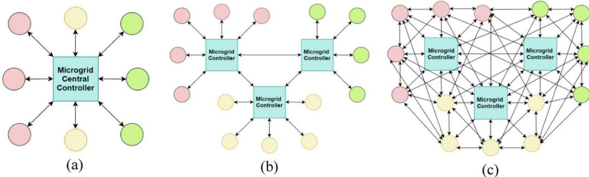
Fig. 4. Various supervisory control approaches for EMS in MG (a) Centralized (b) Decentralized (c) Distributed.
