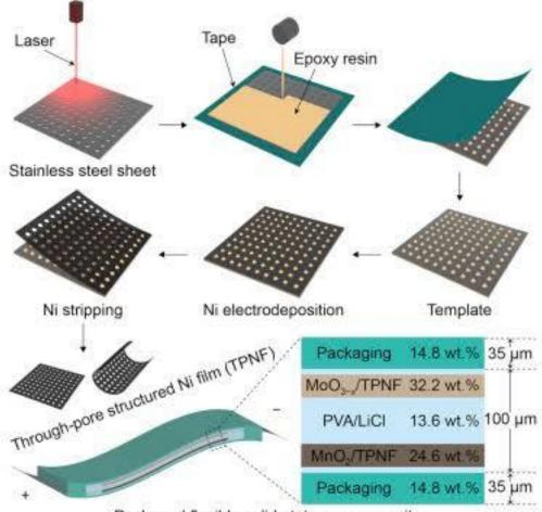
Packaged flexible solid-state supercapacitor
