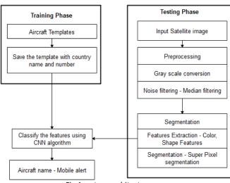
Fig.1 system architecture
