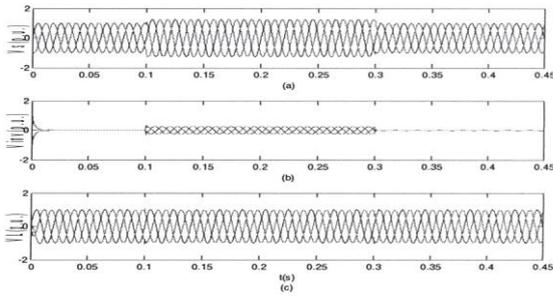
Fig. 11 Three-phase voltages swell: (a)-Source voltage, (b)-Injected voltage, (c)-Load
