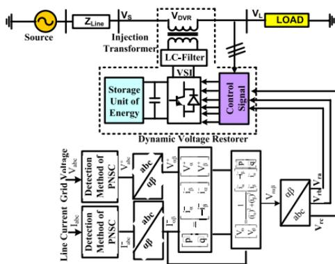
FIGURE 3. Proposed system configuration.
