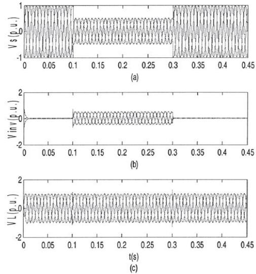
Fig 9: Three-phase voltages sag: (a)-Source voltage, (b)-Injected voltage, (c)-Load voltage
