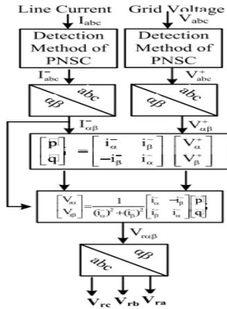
FIGURE 6. Block diagram of the modified PQ method.
