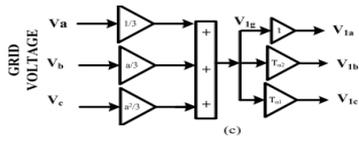
FIGURE 7. (a) Hysteresis voltage controller. (b) Symmetrical components (X: grid voltages or load currents). (c) Extraction method of positive components of grid voltage.
