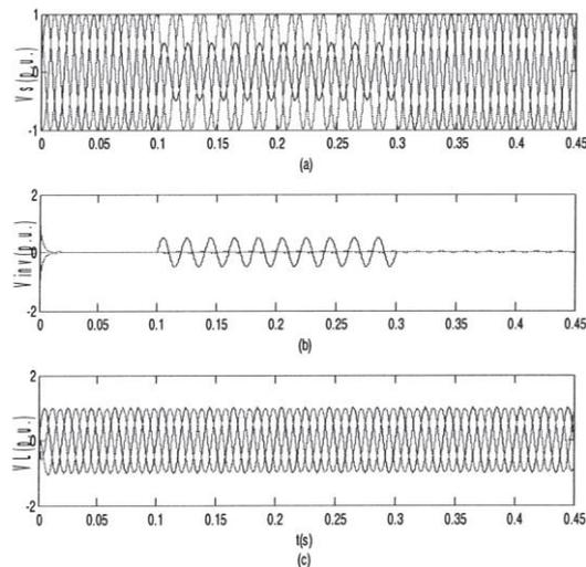
Fig. 10 Single-phase voltage sag: (a)-Source voltage, (b)-Injected voltage, (c)-Load voltage
