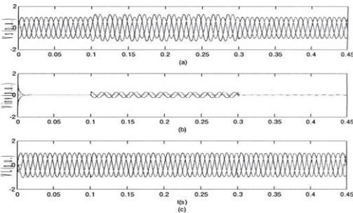
Fig. 12 Two-phase voltages swell: (a)-Source voltage, (b)-Injected voltage, (c)-Load voltage
