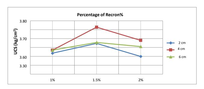
UCS for ALCCOFINE Soil reinforced with Recron-3s Fiber
