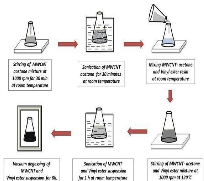
**Fig: 3.1** Schematic view of solution processing technique
